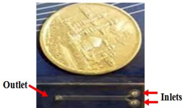
Supplementary Figure2. The designed microfluidic system for the present study. This system was a transparent chip with two inlets and one outlet.
